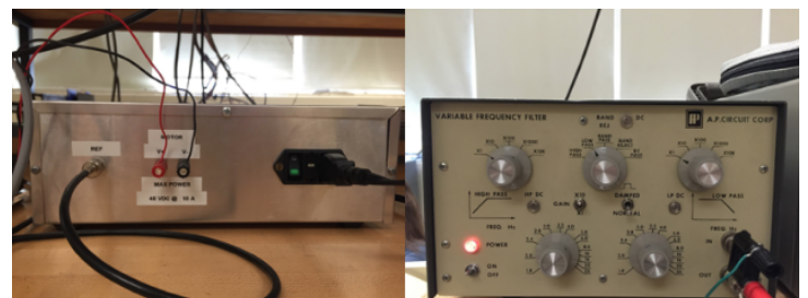
Figure 23: Current Amplifier with 48 V Power Supply (left) and Low-Pass Filter (right).
